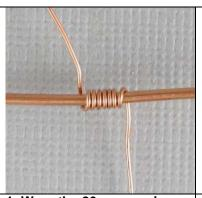
1. Wrap the 26 gauge wire six times around the shorter piece of 18 gauge wire starting 2" from the left end. Wrap the wire away from you.
